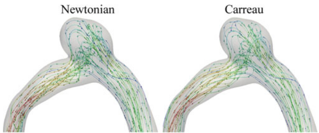
Fig. 15 Particle trace of the Newtonian ( left ) and Carreau ( right ) solutions. Particles are selected at the same location
